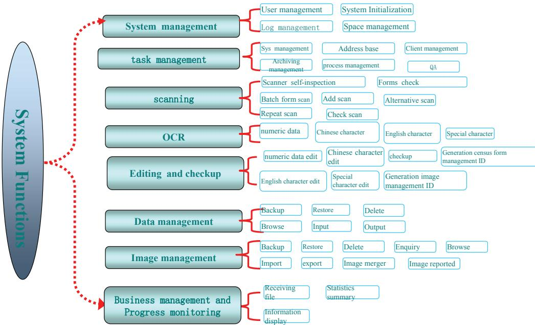
Chart 3 is the function framework of OCR data capture system. It's mainly composed with 8 function modules: system management, task management, scanning, OCR, editing and, checkup, data management, image management, progress monitoring.
